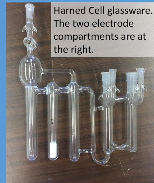
Harned Cell glassware. The two electrode compartments are at the right.
