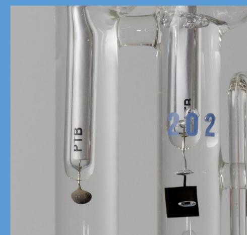
**Above:** Close up of Harned Cell showing Pt H<sup>+</sup> electrode (right) and Ag/AgCl Cl<sup>-</sup> electrode (left)
